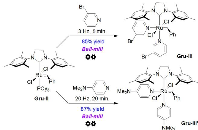
**Scheme 6.** Mechanochemical synthesis of Ru third generation catalyst **Gru-III** and **Gru-III'** via PCy<sub>3</sub>→pyridine exchange.
