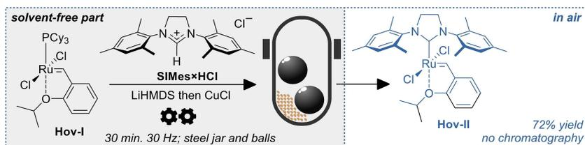
The first solid state synthesis of ruthenium carbene organometallic complexes used as olefin metathesis catalysts is described. It was shown that three key organometallic transformations commonly used in the synthesis of the second and third generations of Ru catalysts in solution—
