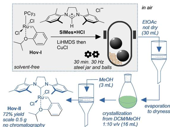
**Scheme 7.** Mechanochemical synthesis of **Hov-II** without using column chromatography. Grey box shows the solvent-free part of the preparation; operations marked in blue were made in air with standard not-dried solvents. Scale of synthesis: 0.5 g. For details see SI.
