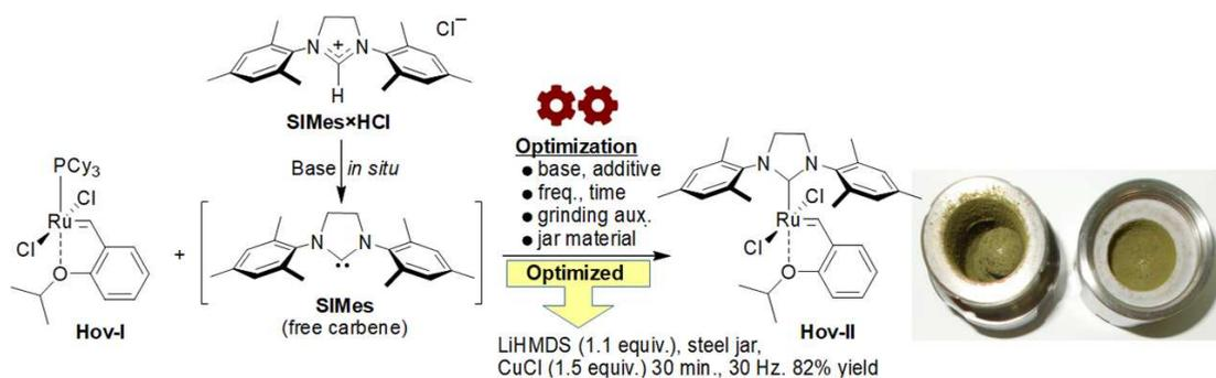
**Scheme 1.** Mechanochemical synthesis of Hoveyda-Grubbs catalyst **Hov-II**. General concept and optimization variables. LiHMDS = lithium 1,1,1,3,3,3-hexamethylidisilazane.
