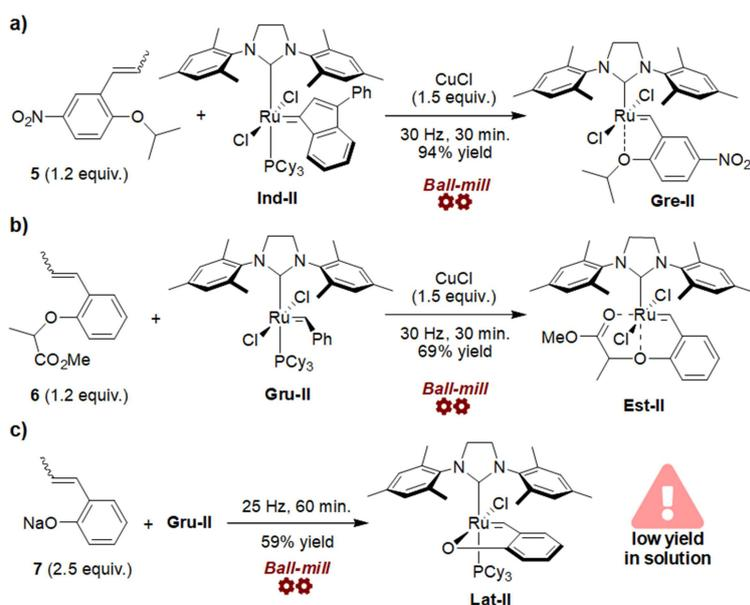
**Scheme 4.** Mechanochemical synthesis of Ru catalysts via alkylidene metathesis-exchange. a) Synthesis of Apeiron Nitro Catalyst (**Gre-II**) b) Synthesis of an 18-electron bis-chelated catalyst (**Est-II**); c) Preparation of Apeiron LatMet polymerization catalyst (**Lat-II**).
