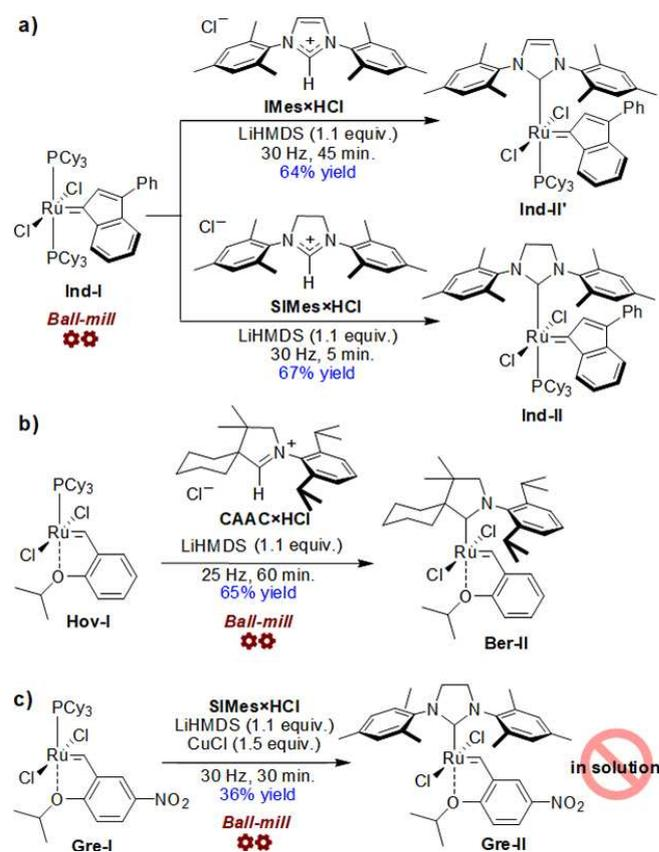
**Scheme 2.** Mechanochemical synthesis of other Ru catalysts via  $\text{PCy}_3$  with NHC (or CAAC) exchange. a) Synthesis of Umicore Grubbs M2 (**Ind-II**) and Evonik Catmetium® RF catalyst (**Ind-II'**); b) Synthesis of Bertrand-Grubbs CAAC complex **Ber-II**; c) Preparation of nitro-catalyst **Gre-II**.
