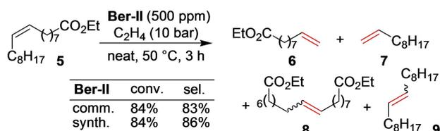
**Scheme 3.** Ethenolysis of ethyl oleate **5** utilising commercial (comm.) and mechanochemically (synth.) prepared **Ber-II**. Conv. = 100 – [(final moles of **5**) × 100 / (initial moles of **5**)]; Sel. = 100 × (moles of **6** + **7**) / [(moles of **6** + **7**) + (2 × moles of **8** + **9**)].
